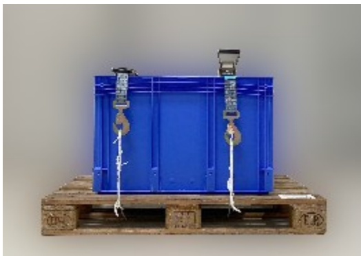
Fig. 3: "Lashing strap" test setup with two five-link textile chain strands
