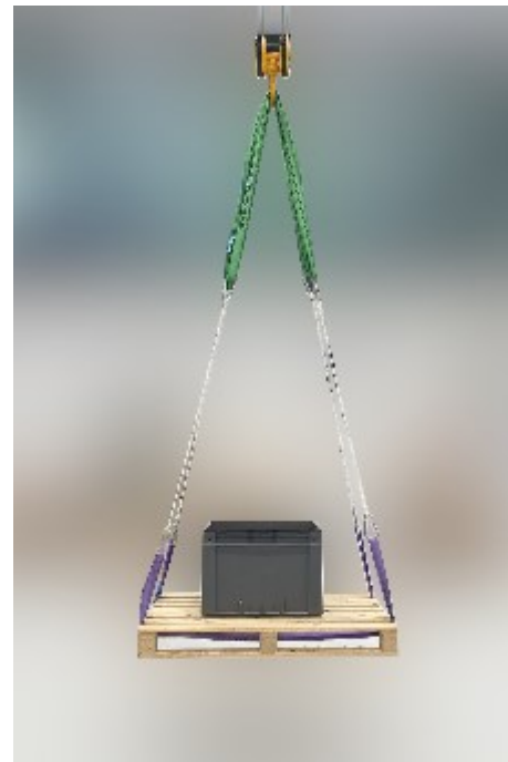
Fig. 2: "Hoist" test setup with four five-link textile chain strands
