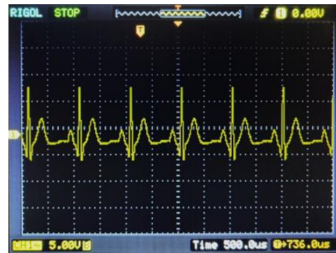
Fig. 7. ECG Signal Waveform on Oscilloscope
