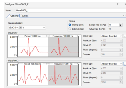
Fig. 4. Setup screen of the WaveDAC8 component in the PSoC5 system
