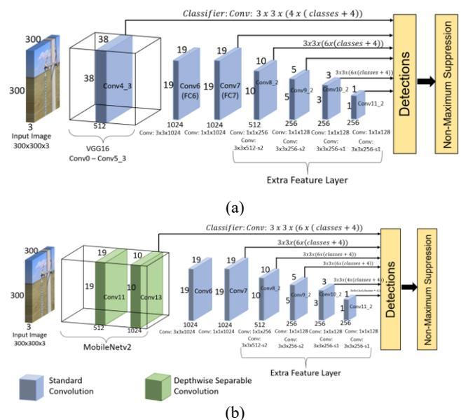
Fig. 1 Network architecture of SSD (a) with standard VGG16 backbone (b) with proposed MobileNetV2
