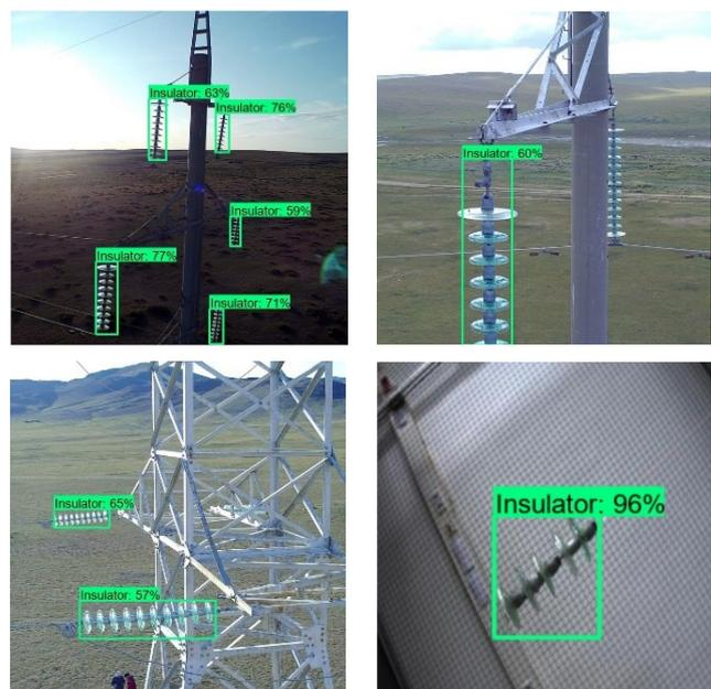
Fig. 3 Power Line Insulator Detection using SSD640
