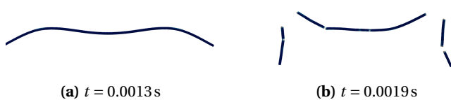
Figure 10 – Break of the beam in the "M-shape" for \dot{F} = 5000 \text{ N/s}
